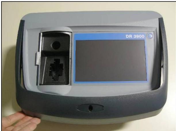
4. Lift the front cover forwards until you can remove it from the instrument.
