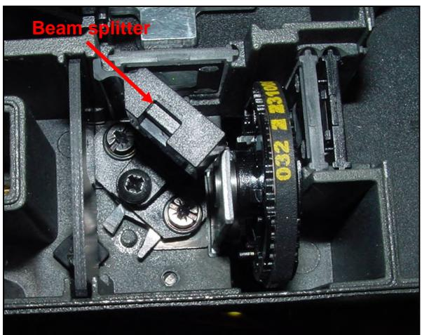
7. The grating is positioned so that from the spectral light band, the green light falls on the exit slit (Photometer → Adjust → Grating refer to [Adjust on page 42](#), menu option "Grating").
