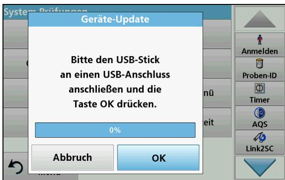
Now insert the VAA608 USB stick and press OK to confirm. The update is carried out automatically.
