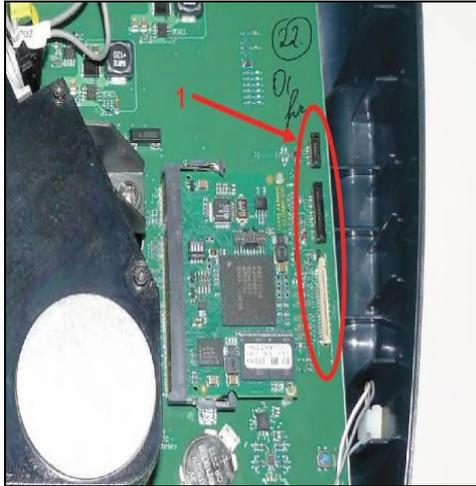
4. Loosen the electrical contacts (1) to remove the display assembly completely; however, in many cases complete removal is not required.
