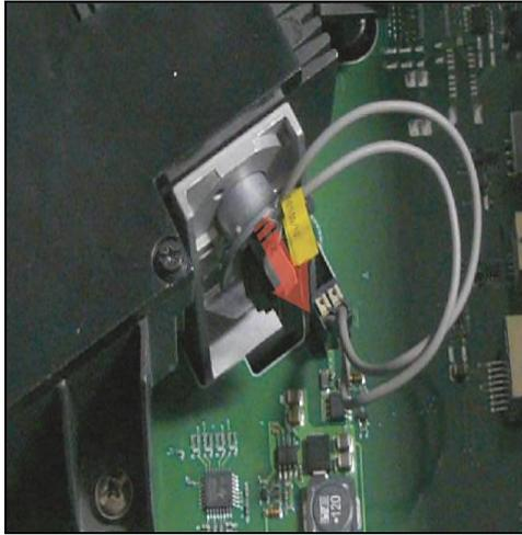
5. Take hold of the plug and pull it and the lamp out of the lamp holder
