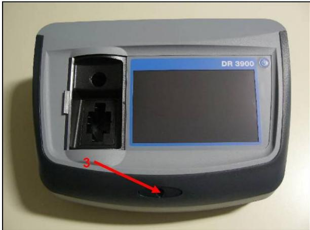
3. Remove the screw (3) underneath the instrument plate.
