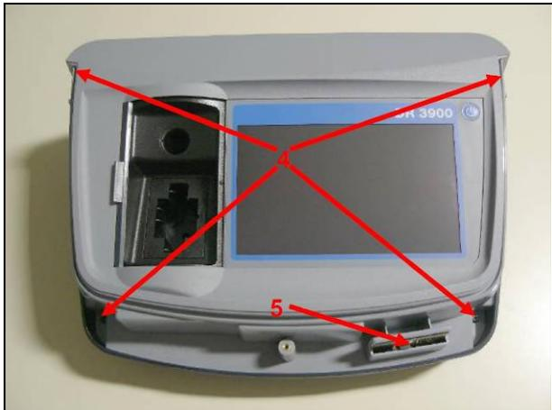
5. Remove the four screws (4) on the top of the housing.
