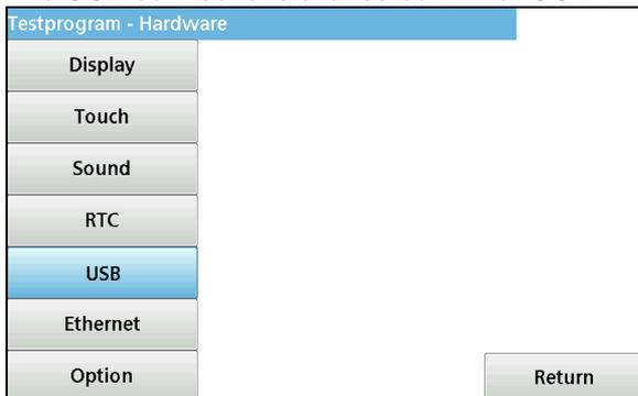
*Note: a USB memory stick (VAA608) and a USB cable type St(A) — St(B) (XLH926) are required for the USB test.*
