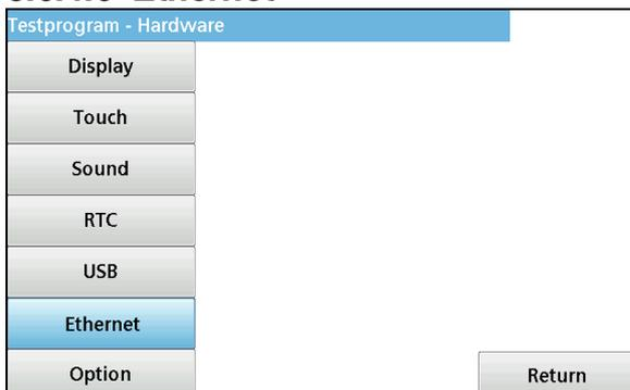
*Note: an Ethernet cable (LZX998) and a PC/Notebook with an Ethernet interface are required for the Ethernet test.*
