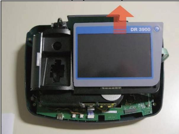
1. Open the instrument (refer to [Open the instrument on page 59](#)).
