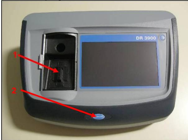
1. Remove the light shield (1) or the cell adapter from the 50 mm cuvette intake.
