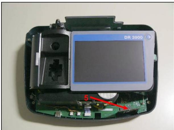
6. Remove the top of the housing by lifting it upwards.
