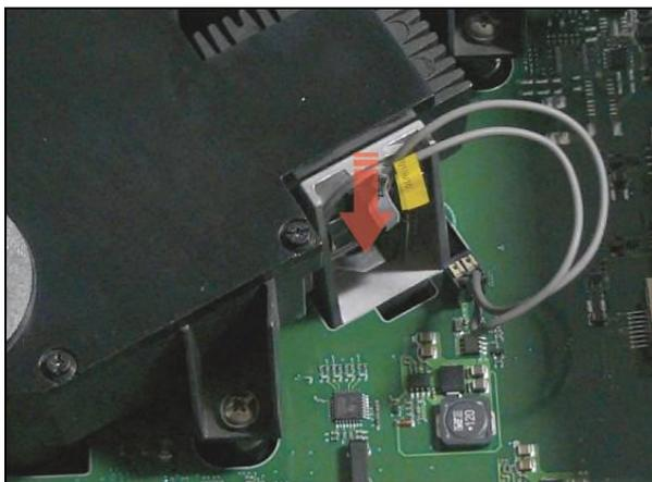
4. Push the terminal slide down to the stop.
