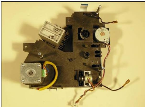
9. To enable better handling of the beam path, it is recommended to attach the 3 spacing bolts back into their threads on the beam path chassis.
